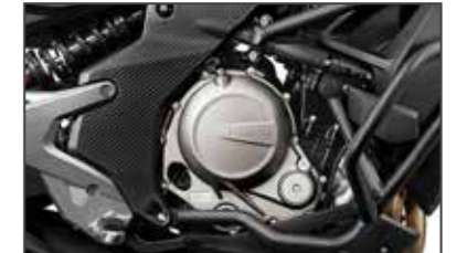
650cc parallel-twin engine
