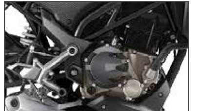
250cc, 4-valve, DOHC engine
