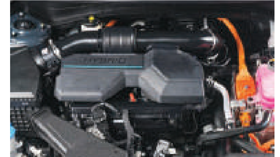
SmartStream G1.6T-GDI HEV Engine Maximum Power: 177 hp Maximum Torque: 265 Nm Motor Maximum Power: 59 hp Maximum Torque: 265 Nm Combined Maximum Power: 227 hp Maximum Torque: 350 Nm Transmission Speed: 6AT
