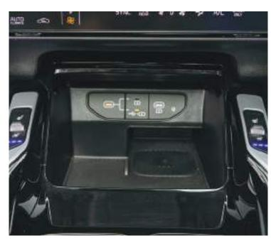
**Wireless Charging Pad**The rubber-lined, wireless charging pad in the center console can quickly charge compatible smartphones.
