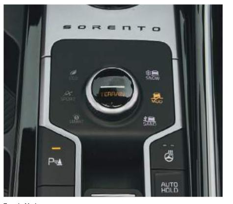
The AWD variant also features Terrain Modes (Snow, Mud, Sand) for enhanced traction and control on challenging surfaces.
