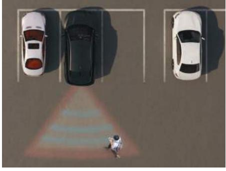
**Rear View Monitor with Dynamic Guidelines**A parking safety features that displays the rear view with parking guidelines using the rear view camera. It provides a rear top view for parking and trailer hooking and offers a continuous rear view driving for enhanced safety.
