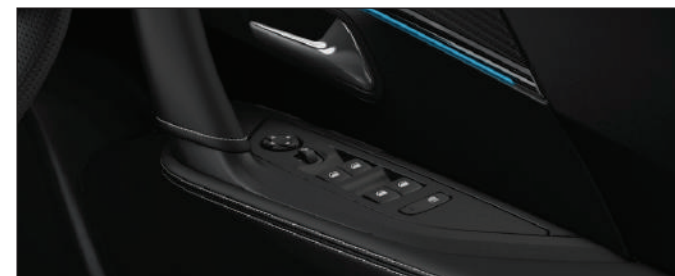
Powered Windows with One -Touch Up/Down & Anti -Pinch
