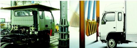
It is the first light duty truck in china to pass ECE R29 top capping test
